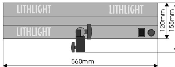
**C110R** is a version of luminaire **C110** with a barndoor covered with light reflecting material.
