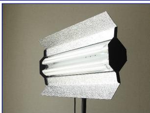
**C110DIM** is a dimmed version of luminaire **C110**. The light flow is adjusted by a potentiometer located on the frame. The adjustment range varies from 10 to 100%. The light flow adjustment helps solving illumination tasks with expedition when there is no possibility to get the light source closer or further away.
